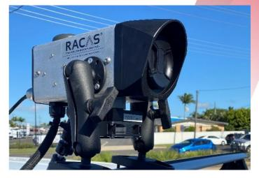
device provides sub-metre accuracy and our new custom engineered roughness device samples every 1/1000th second which means finer resolution, accuracy and repeatability.
